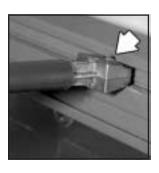
When placing the bows, locate the small notches (arrow) in the side rails.
